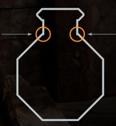
FORCE FROM THE KMR 12 O'CLOCK CLAMP DELIVERS CONSISTENT CLAMPING FORCE THROUGHOUT THE HANDGUARD SURFACE
